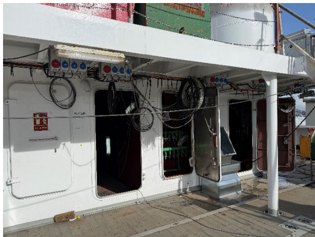
Aft deck with connections for containers and chemical stores + gas bottle store
