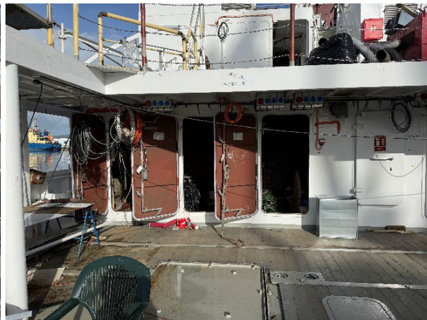
Aft deck with connections for containers and chemical stores + gas bottle store
