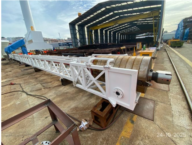
Piston corer with 30-metre core barrel and piston ladder
